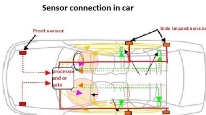
Figure: 5.1 Vibration Sensor connection in car
